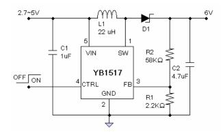
Figure 5: TFT Panel Power Application Circuit
