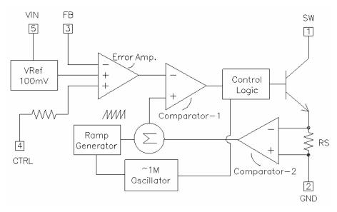
Figure 3: YB1517 Block Diagram
