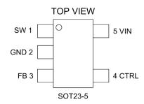
Figure 3: YB1517 Pin Configuration
