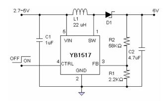
Figure 2 : DC-to-DC Converter
